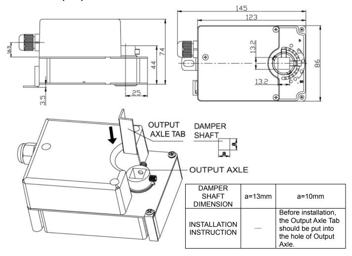
Note: Only suitable for  $13 \times 13$ mm or  $10 \times 10$ mm foursquare damper shaft. Other sizes of aluminum gaskets can be made when the Damper Shaft dimension "a" is smaller than 10mm.
